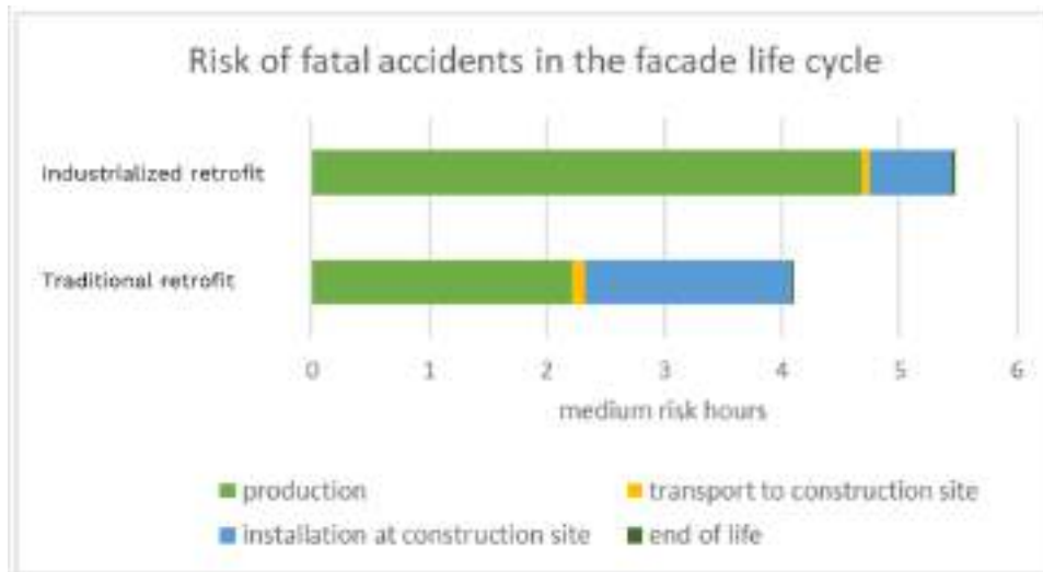
Figure 49: Life cycle contribution to risk of fatal accidents – traditional vs industrialized facade renovation
