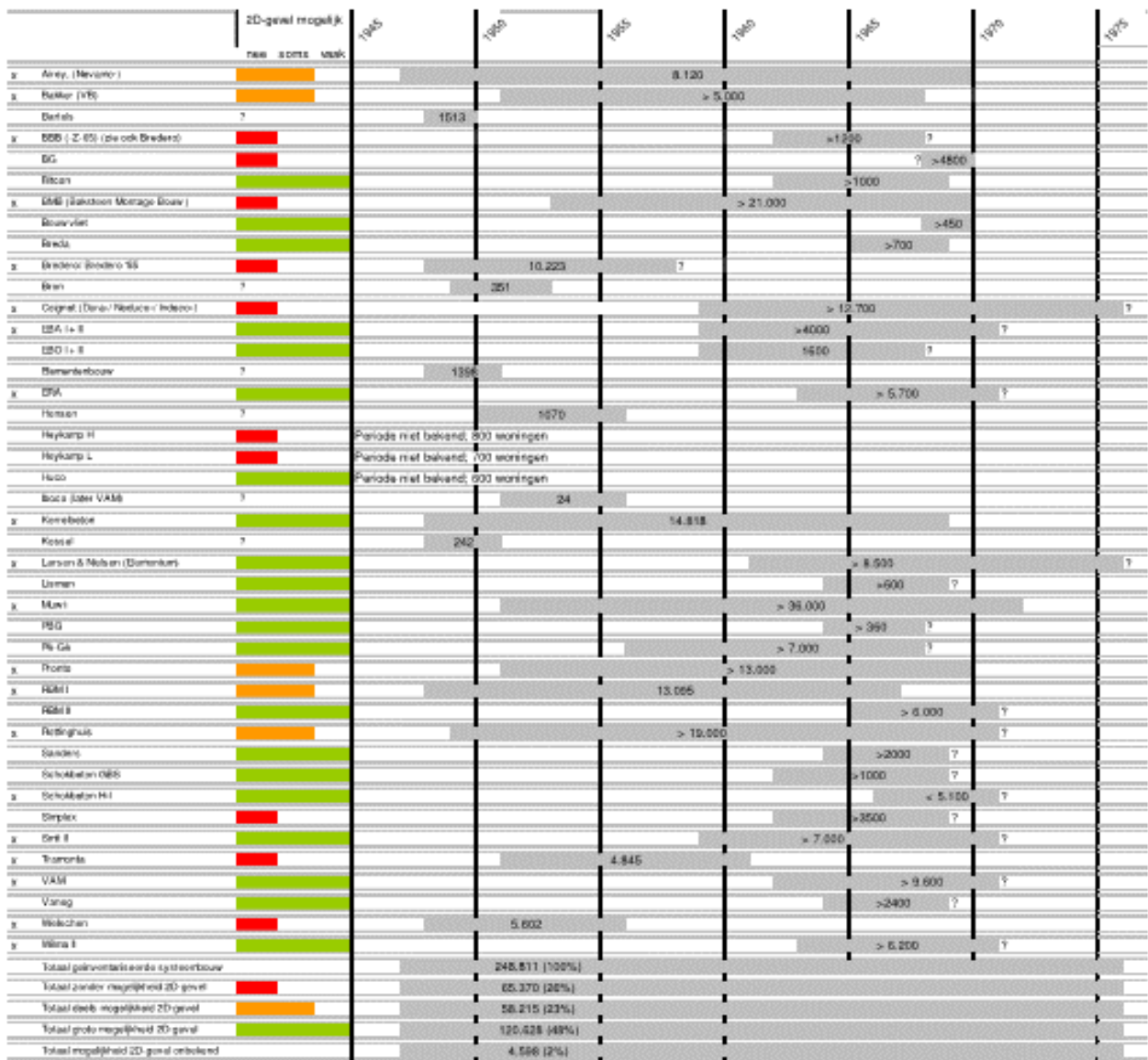
Figure 35 Overview of the Dutch post-war prefab system building flows and its potential for prefab renovation.
